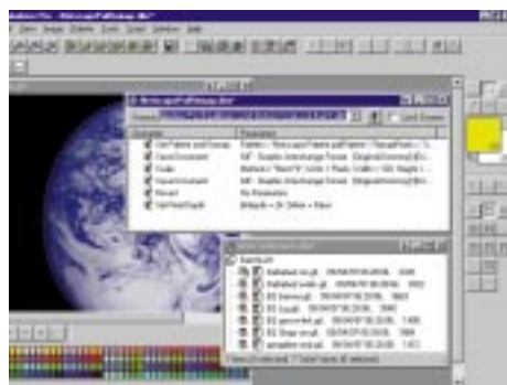
Setting up automated processing couldn't be easier. The script in the top window is applied to all the images in the batch list in the lower window
